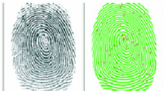
Fig. 2 The image obtained from the reader (left) and image processed using the method 'minutiae'
